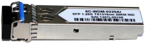
1000Base-BX WDM Singlemode (TX 1310 nm – RX 1550 nm)
