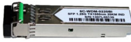
1000Base-BX WDM Singlemode (TX 1550 nm – RX 1310 nm)
